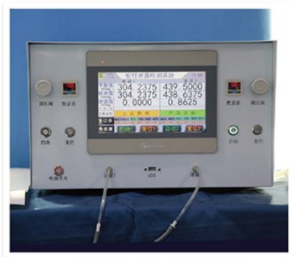
Bladder Leakage Testing 气囊漏气测试
